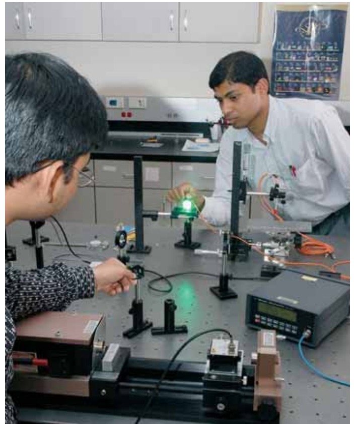
Graduate student Gopalendu Pal (left) aligns a laser while Dr. Kunal Mitra measures optical signals from phantom tissue samples.
