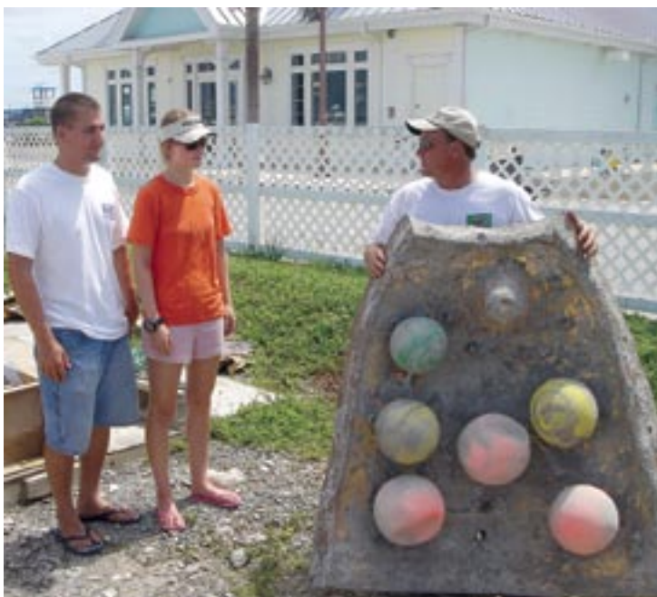
Ocean engineering graduate students Doug Bowlus and Ashley Naimaster learn mold construction techniques for fabricating Reef Ball units from Larry Beggs, president of Reef Innovations, Inc.
