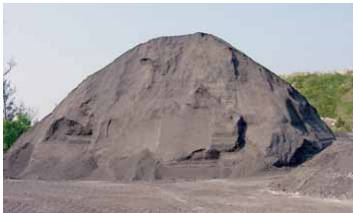
Large RAP piles, like the one above, result from millings that cannot be used by contractors in new hot mix asphalt—an increasing problem throughout the state.
